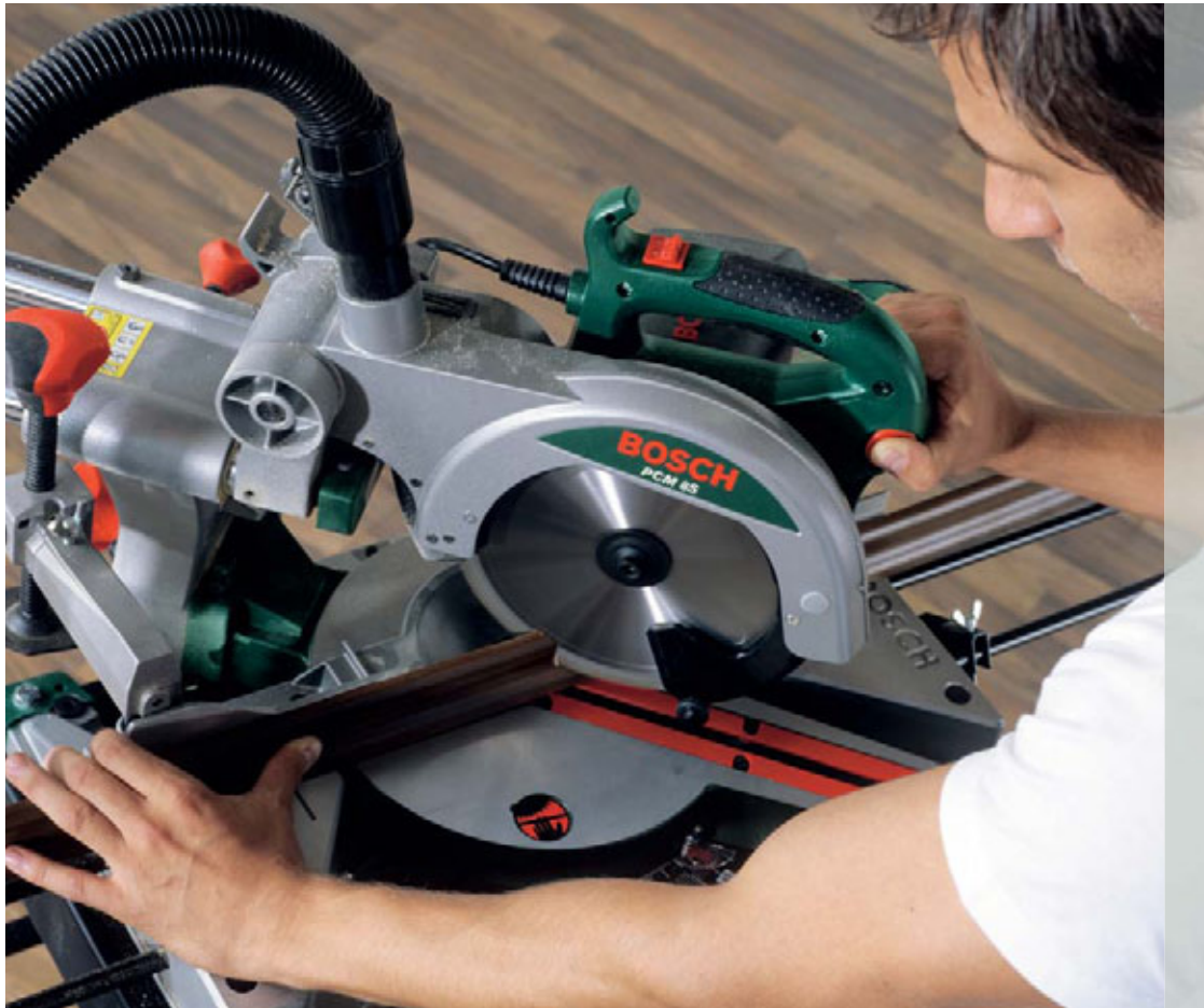
A typical case for a mitre: to make it possible to put the skirting boards flush against each other in corners, they are mitre-cut using the compound sliding mitre saw.
