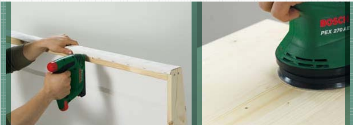
6. Cover the canopy frame with canopy fabric
