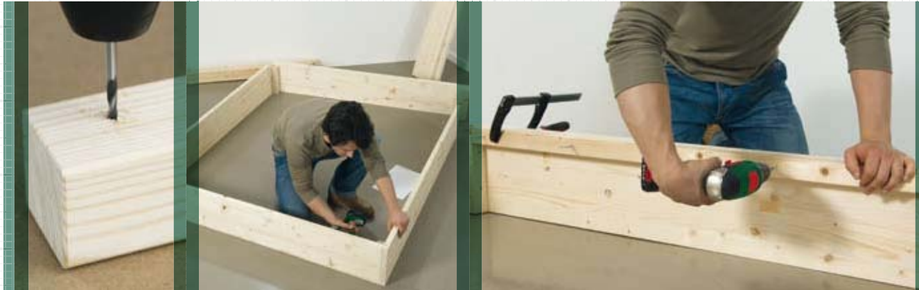
1. Join the surrounds with the screw strips
