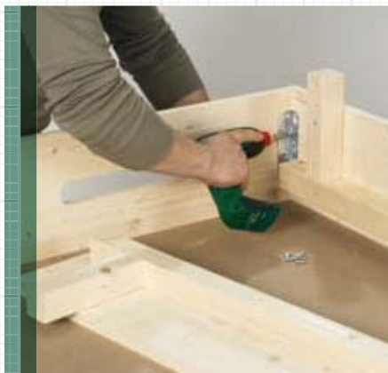
2. Base frame: Mount the legs and square timbers
