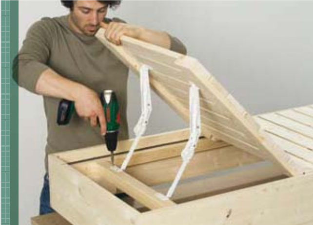
5. Fasten the seat back supports and simultaneously fit the attachment strip
