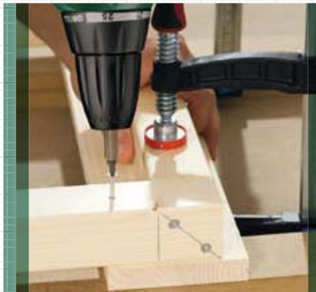
2. Join the base frames with the frame surrounds
