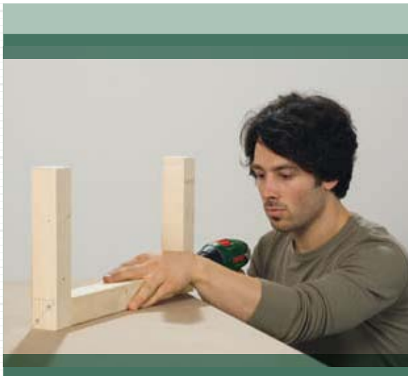
1. Fasten together the legs and cross connectors to form base frames
