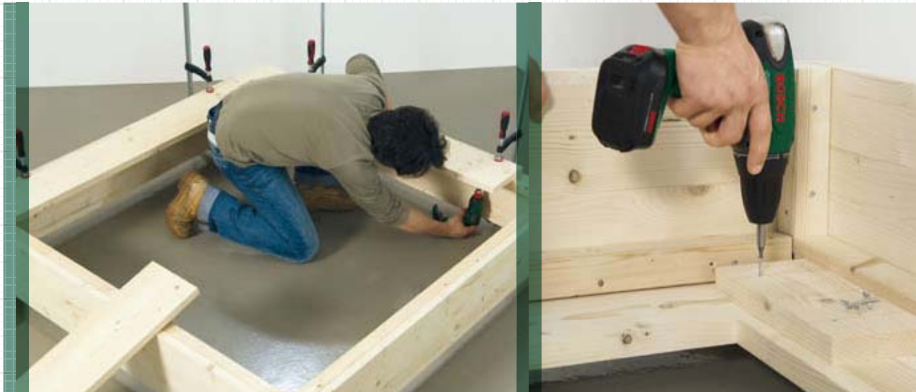
2. Join the bench boards with the frame
