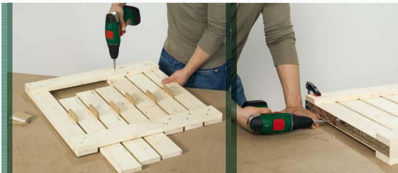
4. Fasten the slatted frame parts and connect them with the piano hinge
