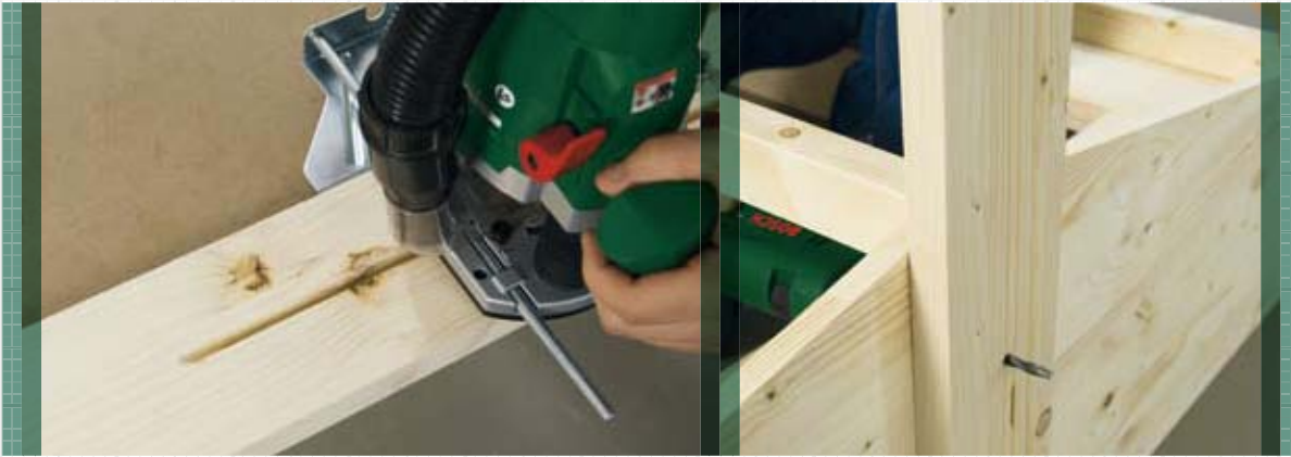
5. Prepare the canopy supports and join them to the sandpit
