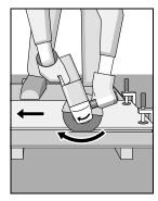
The machine must always work in an up-grinding motion. Otherwise, the danger exists of it being pushed **uncontrolled** out of the cut.
