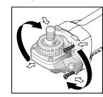
The machine head can be rotated with respect to the machine housing in 90° steps. In this manner, the On/Off switch can be brought into a more convenient position for special
