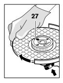
Lock the grinder spindle with the spindle lock button **1**. To tighten the quick-clamping nut, firmly turn the grinding disc in clockwise direction. Therefore, observe the permissible **rotational/ circumferential speed** on the label of the grinding tool.
