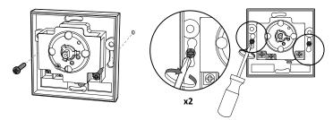
5- Use the two opened areas in order to pass the wires from the wall/back box.
