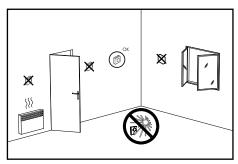
Important: The thermostat measures the temperature of the place where it is installed. It does not take into account the temperature differences that may exist between different locations in the house if the temperature is not uniform.
