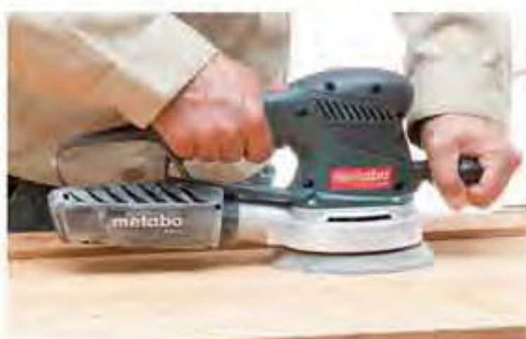
Suitable for general curved and flat sanding applications
