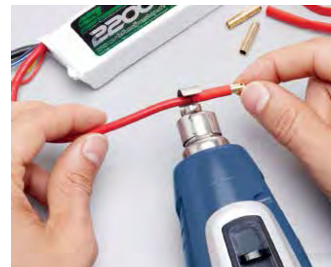
Heat-shrinking. Secure standing for hands-free work.
