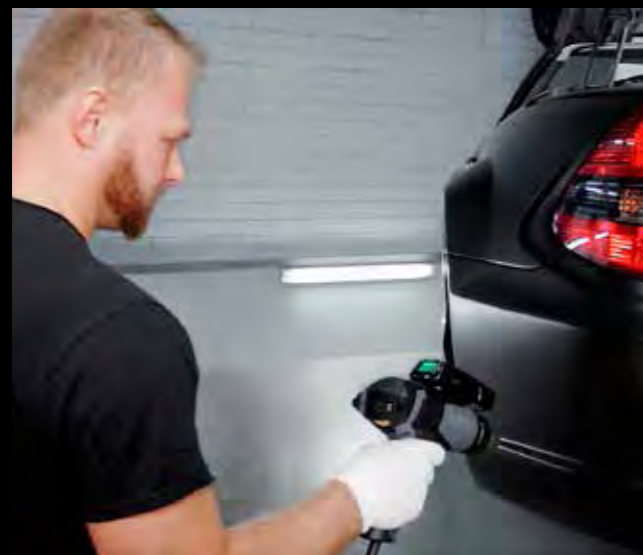
Hot air and temperature measurement with one hand while car wrapping.
