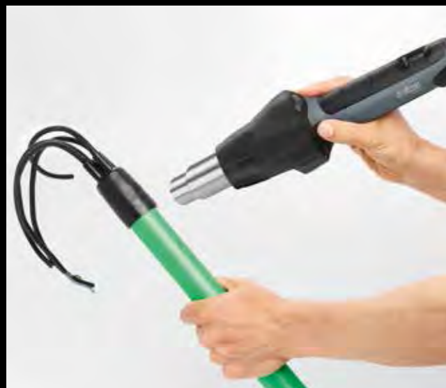
Industrial heat-shrinking for wiring harnesses.
