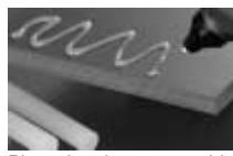
Place the glue on one side by squeezing the trigger. Press the glued parts firmly together. After approx. 2 mins. the connection is solid.
