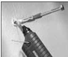
Losse deuvels vastzetten.
