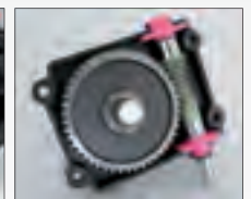
Enclosed worm drive with angular metal gears
