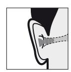
3. The plug will then be correctly positioned in the ear canal ensuring it offers maximum hearing protection.
