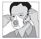
Ensure respirator fits secure and comfortable. To fasten respirator pull strap at either side of the buckle.
