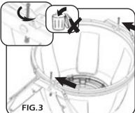
Unscrew both screws holding temporary axles (Fig.3, two places)
