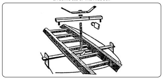
Assemble components as shown above to make two rack clamps (padlock not included). Always use rack clamps in pairs, one at the front and one at the rear of the vehicle.
