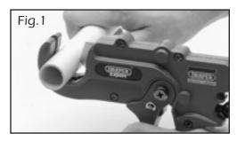
2. Squeeze the trigger to operate the ratchet action, until the material is cut.
