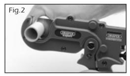
3. Push the button to release and retract the blade.
