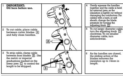
4 Gently squeeze the handles together and the cable is held by external jaws, as the insulation is lightly cut without damaging the conductors. For cables with a hard, or soft sheath, change the blade pressure by turning the adjusting knob
