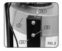
Pass the two (M8 x 45mm) bolts (13) through the handle (8), the upright (24), the spacing block (24.1) and the collection bag ducting (4) and secure in place with the (M8) nuts (12).
