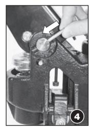
Secure the axle pin by locating the dowel pin (soft face hammer required).
