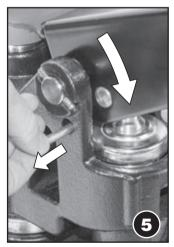
Push the handle down and remove the pump securing pin.
