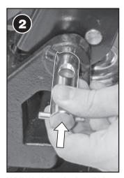
Whilst holding the handle in place slide the axle pin through the handle.
