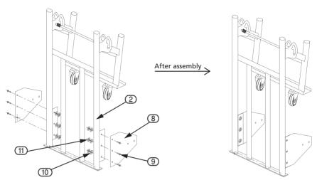
Step 2: Plug the Movable Toe Plate (12) into the Frame (2) in the way shown below.
