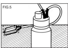
When the float switch reaches the minimum level it will automatically switch the pump off.
