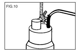
If pumping water from a sandy or muddy floor bed, the pump can be suspended using a rope or chain (not supplied) fixed to the handle. DO NOT use any of the electrical cables for this purpose.
