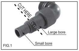
**NOTE:** The adaptor can now only be used with a large bore hose and cannot be used with a smaller bore hose.
