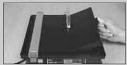
For mitre cuts, raise the hinged section of the table to the required angle (22.5° or 45°)
