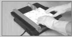
Maintaining an even pressure, hold the tile against the cutting guide and push steadily through the cutting blade. When the cut is complete, switch off the machine.
