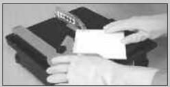
Switch on the machine and while holding the tile firmly in position, push the mitre guide steadily along the rip guide, feeding the tile through the cutting blade.
