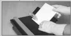
Switch on the machine and feed the tile through the cutting blade. When the cut is complete, switch off the machine.
