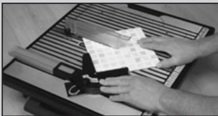
Switch on the machine and while holding the tile firmly in position, push the mitre guide steadily along the rip guide, feeding the tile through the cutting wheel. When the cut is complete, switch off the machine.
