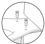
For top fix, insert the rubber plugs into the holes in the toilet pan.
