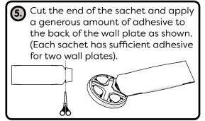
Sufficient adhesive must be applied to give a uniform thickness of approximately 1.5mm when the wall plate is positioned against the wall.
