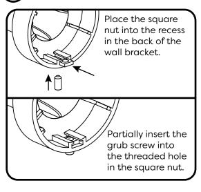
Once the Flexi-Fix wall plates are secured to the wall, place the Riser Rail brackets over each of the Flexi-Fix wall plates and secure by tightening the grub screw with the hex key provided.
