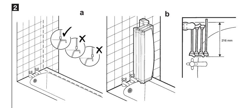
Position the screen so that it rests along the inner edge of the bath (a). It is advisable that the screen is fitted so that it will fold into the bath (b) Check the measurement above (4 and 5 panel version) to ensure you have sufficient space
