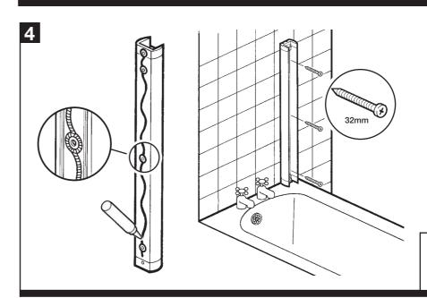
Apply silicone sealant to back of wall channel as shown. Fix wall channel to wall using the 32mm screws.
