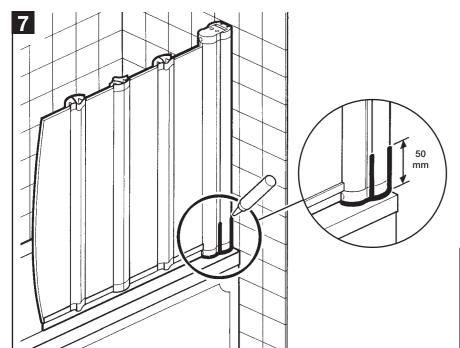
Apply silicone sealant to the outside of the screen where shown.
