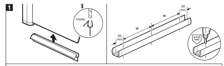
Fit the seal to the bottom of the bathscreen ensuring the seal 'flap' is on the inside of the screen, trim to length if required.
