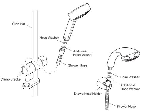
**Note!** The Mira Universal Shower Hose has been supplied with 2 extra hose washers, if the hose should leak following installation, simply add additional washers.
