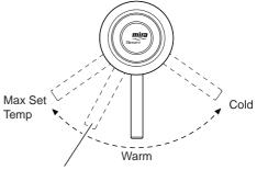
Temperature Overide approximately 5°C below Max Set Temperature.
