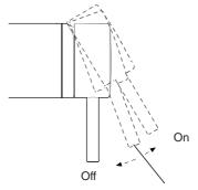
Mid Flow Overide - Reduces water flow by up to 30% (dependant on inlet pressures) and can be overridden by increasing flow to full.
