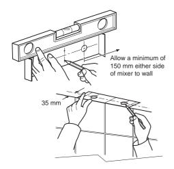
For solid walls drill the holes for the backplate with a 6 mm diameter drill and insert the wall plugs.
