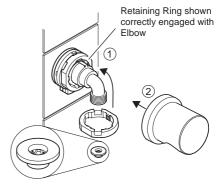
**Note!** For high pressure systems (above 0.5 bar) make sure that the flow regulator (supplied) is fitted inside the elbow in the orientation shown.
