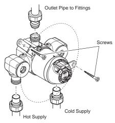
**12.**Remove the two shroud screws and refit the building-in shroud to the mixer.
