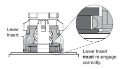
13.Make sure that the two cartridge inlet seals are fitted and carefully push the cartridge into the body, aligning the cartridge lugs into the body slots.
