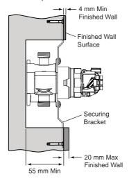
**3.** Fit the securing brackets to the mixer with the bracket securing screws.
