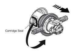
8. Use the 2.5 mm hexagonal key or a suitable sized screw driver to push the hinge pin from left to right, releasing the lever insert (refer to illustration).
