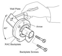
**12.**Remove the assembly from the wall and separate the backplate from the wall plate.
