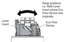
12.Repeat the procedure to refit the lever insert making sure that it re-engages correctly with the cartridge.
