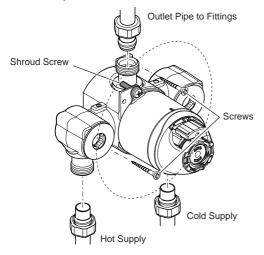
12.Connect the outlet pipework and install the RAC assembly or BIR assembly, before continuing with the installation of the mixing valve.
