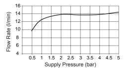
Typical flow rates on low pressure systems (0.1 to 1 Bar) without flow regulator fitted - Mira Element SLT with L14A Shower Fittings
