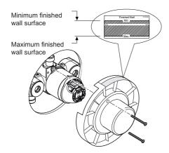
13.Using the 'Finished Wall Indicator' on the building-in shroud as a guide, finish the wall, e.g. tiles.
