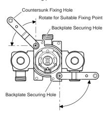
**Note!** Securing Brackets shown in preferred position to allow the Compression Nuts to be tightened.
