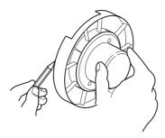
Mark the routes for the supply pipework at 108 mm centres (Hot - Left, Cold - Right).
