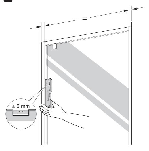
(a) Centralise the door frame within the wall channels, making sure that the door frame is square.
