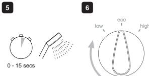
Water flows freely within a few Turn power control to Eco. seconds, temperature remains cool.
