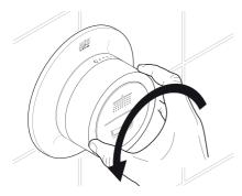
Adjust the temperature indicator in accordance to the table below to set the desired maximum temperature.
