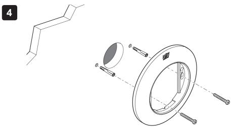
Fit the backplate to the wall in the orientation shown using the fixing screws (supplied). Tighten by hand, do not over tighten.
