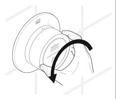
Adjust the temperature indicator in accordance to the table below to set the desired maximum temperature.
