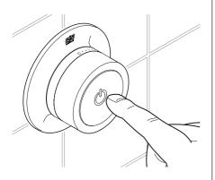
Hold down the On/Off Button for 10 Seconds approx. until the Temperature Indicator light pulses on/off.
