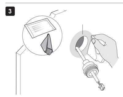
Using the cleaning wipe (supplied) clean the surface around the mounting hole.
