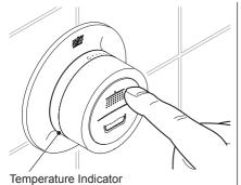
Hold down the Overhead Shower Button (top half) for 10 Seconds approx. until the Temperature Indicator light pulses on/off.
