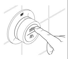
Press the Overhead Shower Button to set the maximum temperature. The temperature indicator light will flash twice to confirm the setting has been completed.
