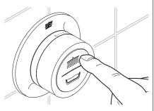
Press the Overhead Shower Button to set the maximum temperature. The temperature indicator light will flash twice to confirm the setting has been completed.
