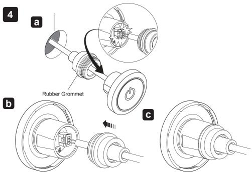
Connect the cable to the back of the ON/OFF button.
