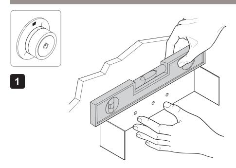
Position the installation template (supplied) at the position on the wall where you intend to install the interface. Make sure that the template is level.
