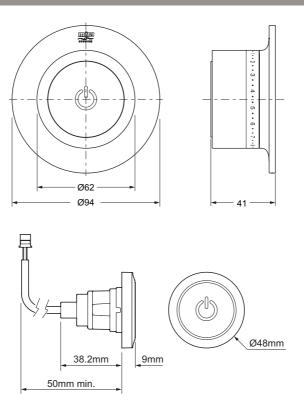
Refer to Digital Mixing Valve Installation guide for schematic.
