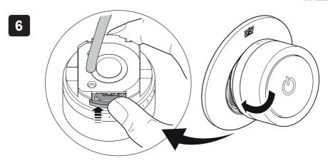
Locate the top of the interface in the backplate and press down on the bottom button as you install in position.
