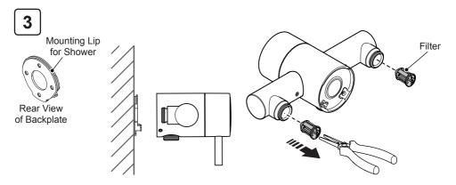
Remove the shower unit from the wall. The filters are retained in the elbows, remove them using a suitable tool and inspect for damage or debris blockage.
