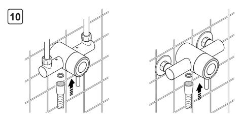
Install the shower's outlet fittings, see 'Shower Fittings Installation & User Guide' for instructions. Fit the shower hose with a 15mm rubber washer. Turn on the water supply and test the shower.
