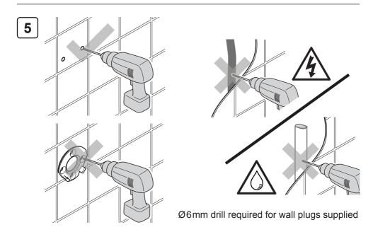
Drill the fixing holes for the backplate.
