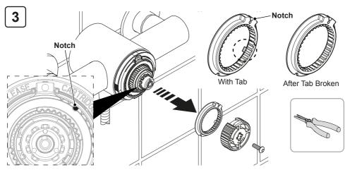
Remove the hexagonal screw and remove the hub and the temperature trim. Break off the tab on the temperature trim to adjust the temperature.
