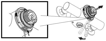
Lever the cartridge out using a suitable flat blade screwdriver. Continue to lever the cartridge until it can be removed easily by hand.
