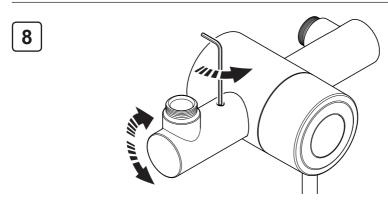
To adjust the shower unit for falling/rising water supplies, loosen the hexagonal screws and rotate the elbows. Re-tighten the screws to secure the elbows, ensuring the elbows are pushed firmly back against the body.
