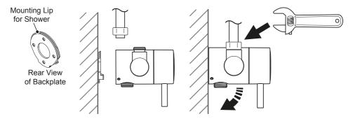
Fit the shower unit over the backplate and secure to the pipework. Avoid damage to the chrome finish when tightening the compression nuts.
