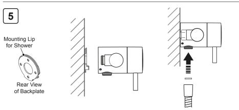
Refit the shower unit to the wall and the pipes. Reconnect the shower hose, then restore the water supplies and check for leaks.
