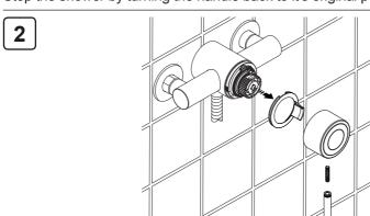
If this temperature needs to be either warmer or cooler, carefully remove the lever, the grubscrew, the handle and the bearing.
