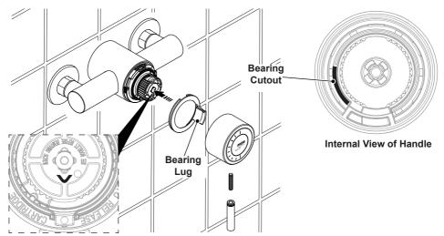
Refit the bearing ensuring the lug is in the bottom right hand corner. Replace the handle ensuring that the arrow on the yellow hub is pointing downwards, and ensuring the cutout on the inside of the handle matches up with the lug on the bearing. Refit the grubscrew and the control lever.
