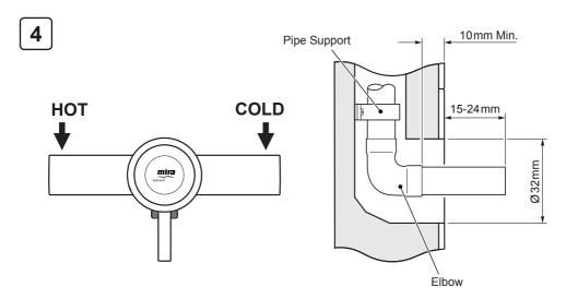
Fit the supply pipework, *HOT* and *COLD* supplies can be reversed. Any recessed inlet pipes must extend 15-24mm from the finished wall surface, and be square to the wall.
