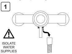
Isolate the water supplies. Turn the shower on and off to relieve pressure. Disconnect the hose from the shower unit.
