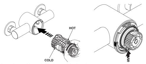
Insert the cartridge and slide the snap ring into place.
