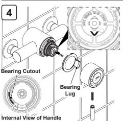
Refit the bearing, ensuring the lug is in the bottom right hand corner. Replace the handle, ensuring that the arrow on the yellow hub is pointing downwards. Ensure that the cutout on the inside of the handle matches up with the lug on the bearing. Refit the grubscrew and the control lever.
