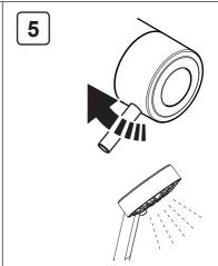
Check the maximum showering temperature by turning the handle fully clockwise.
