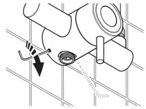
Secure the shower unit to the backplate. **DO NOT** overtighten the screws.
