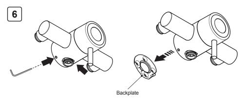
Loosen the two hexagonal screws and remove the backplate from the shower unit.
