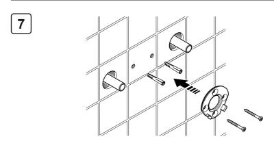
Fix the backplate to the wall using, 2 x No. 8 x 11/4" screws and wall plugs (supplied).
