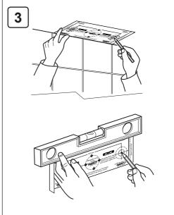
Use the template provided to mark the positions of the pipes and fixing holes (choose either the vertical pair or the horizontal pair).
