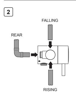
Determine the route for the supply pipes. For rear inlet, use an elbow fitting. We recommend a falling supply to prevent air locks.
