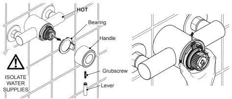
Carefully unscrew the lever and the grubscrew and remove the handle along with the bearing. Unclip the snap ring as shown.
