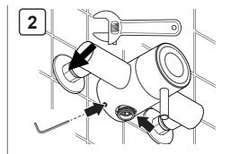
Loosen the hexagonal screws as shown and both of the compression nuts. Avoid damage to the chrome finish when loosening the compression nuts.
