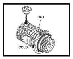
Remove the bung from the top of the cartridge. Place the bung in the opposite side.
