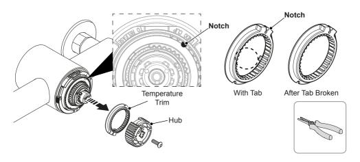
Remove the hexagonal screw and remove the hub and the temperature trim.
