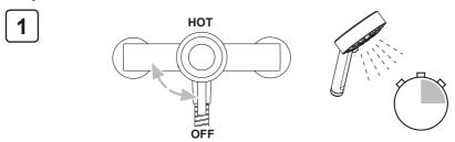
Turn the handle until water starts to flow, allow a few seconds for the temperature adjustment to take full effect, check that the product is flowing cold water.
