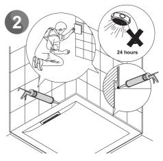
Tile the walls down on top of shower tray. Apply silicone sealant in accordance with the manufacturer's instructions to seal the shower tray to the tiled wall surface.
