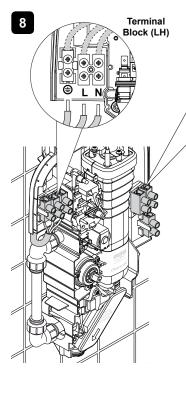
Ensure the earth bonding complies with relevant regulations.
