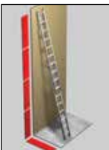
Correct Angle for Climbing a Ladder
