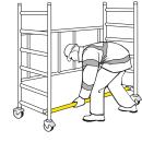
Fit the four spring interlock clips supplied with the extension pack. Expand the clips over the top of the base unit uprights and then slide down to engage the pin on the clip into hole in the upright.
