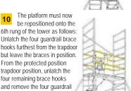
Descend the tower. The platform should now be repositioned in the tower by moving it from 8th rungs to the 6th rungs (the top rungs of the base frame)
