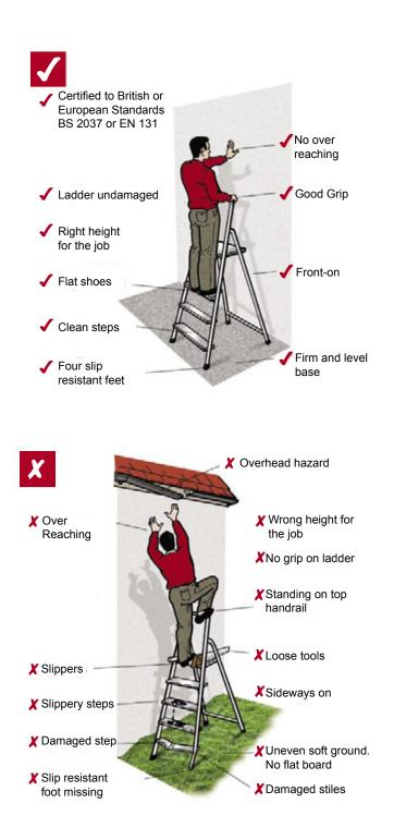
A step ladder is an important piece of equipment. Used correctly and safely a Youngman step ladder will provide many years of reliable use.
