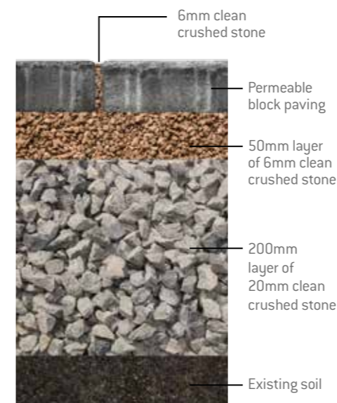
3. Prepare your laying course using 50mm of 6mm clean crushed stone. Only light compaction required.
