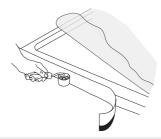
Note! With some types of waste unit, it may be necessary to form a keyhole shaped cutout in the ply using a jigsaw. This will make access to the waste unit easier. Note! Some shower trays have a protective film (indicated by a label on the surface) which MUST now be removed. Undertake a final inspection of the shower try at this stage. DO NOT PROCEED IF NOT SATISFIED.
