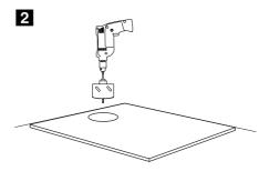
Place the shower tray **(a)** in position on the floor (ensuring surface is level) and mark the perimeter on the floor including an area outside the perimeter for access to connect plumbing (as dictated by the installation location) after the shower tray has been installed.
