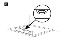
Mix fine sand, cement and a cement additive in accordance with the manufacturers instructions to a workable mix to cover the total area under the tray. Trowel to a thickness suitable to allow leveling and full support of the shower tray.
