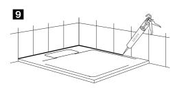
Fit waste cover **③**. The shower tray and all connections **MUST** now be checked for water tightness, flow and adequate drainage over the entire area with the waste cover **④** in position.
