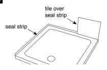
Using a small roller or other appropriate tool roll the seal strip so that it attaches firmly to the edge of the tray removing any bubbles or creases, paying particular attention to the corners.
