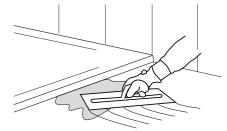
When the cement has set, make connection between the shower tray and waste piping. The shower tray and all connections **MUST** now be checked for water tightness, flow and adequate drainage over the entire area.
