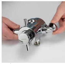
Adjust the Aspire valve inlet elbow centres to suit (between 148mm and 155mm)
