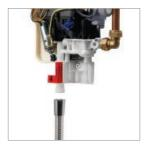
Ensuring the electric supply remains isolated turn on the water supplies. Push the solenoid piston up until water runs through and out of the hose for a few seconds before releasing the piston.
