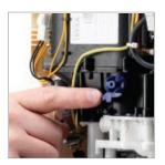
Hold the cover next to the shower unit on the wall and carefully attach the two solenoid connectors. Place the solenoid connector block into the saddle within the shower unit and neatly tuck the wires into the recess provide.
