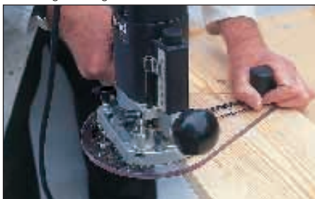
...and gives greater control over the router when moulding the edge of a board
