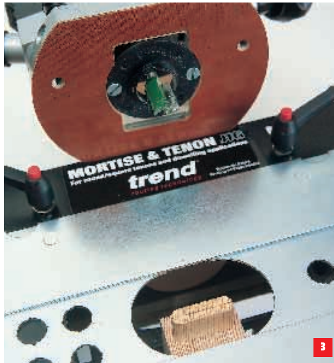
The resulting tenon. Note rounded ends
