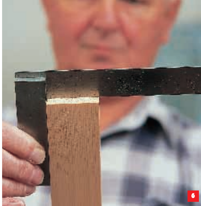
A tenon piece being checked for square after 'shooting'
