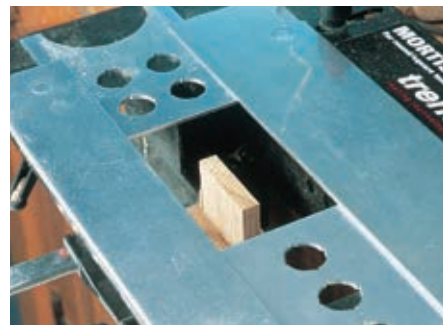
Square tenons can be cut by simply reversing the guide plates.
