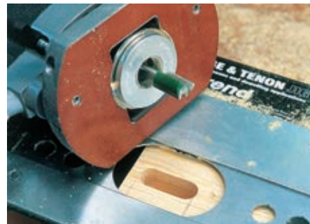
The rounded ends of the mortice perfectly match those of the tenon.
