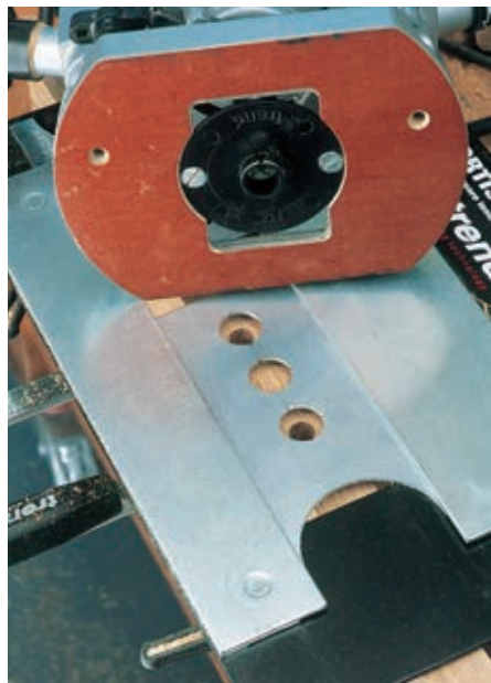
The jig can also be used for making dowel joints.
