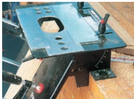
Compound angles are also possible as the front of the jig hinges forward.
