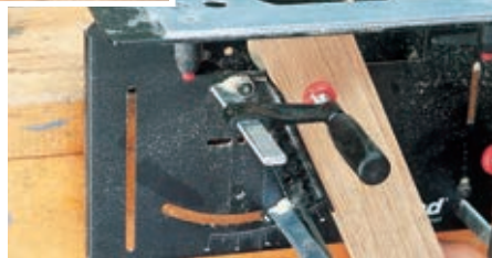
Angled tenons are equally simple as the fence will tilt up to 45°.
