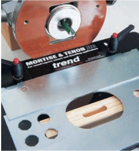
Mortise being cut after swapping bush and cutter combination
