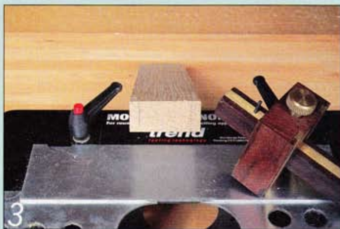
3 Marking the end of the timber to be tenoned
