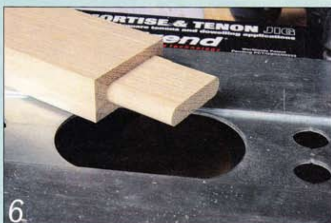
6 Several shallow passes will produce a nice clean tenon time after time
