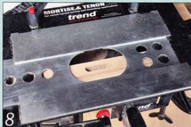
8 Several shallow cuts will soon have the mortise cut to depth
