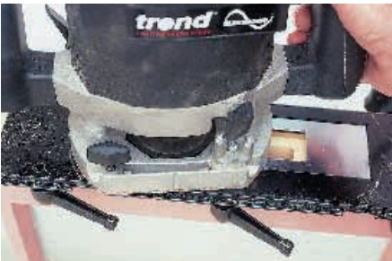
Cutting the mortice.
