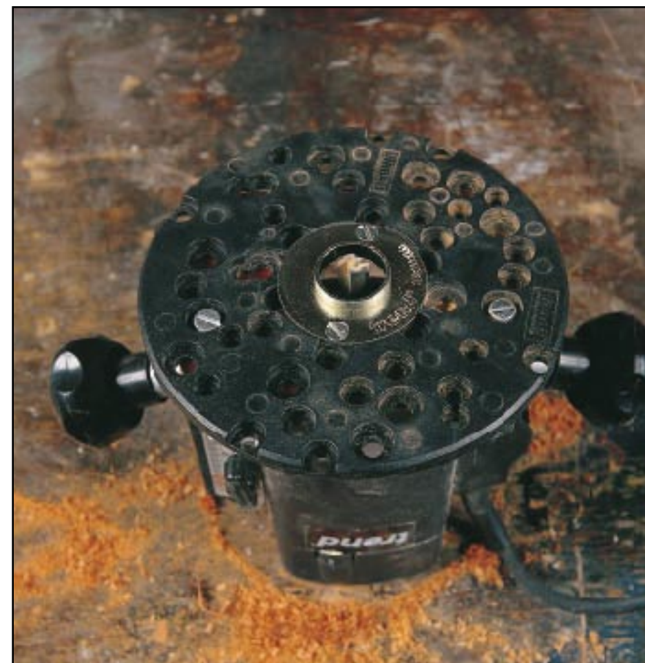
◀ A Trend guidebush and cutter installed after centring the Unibase
