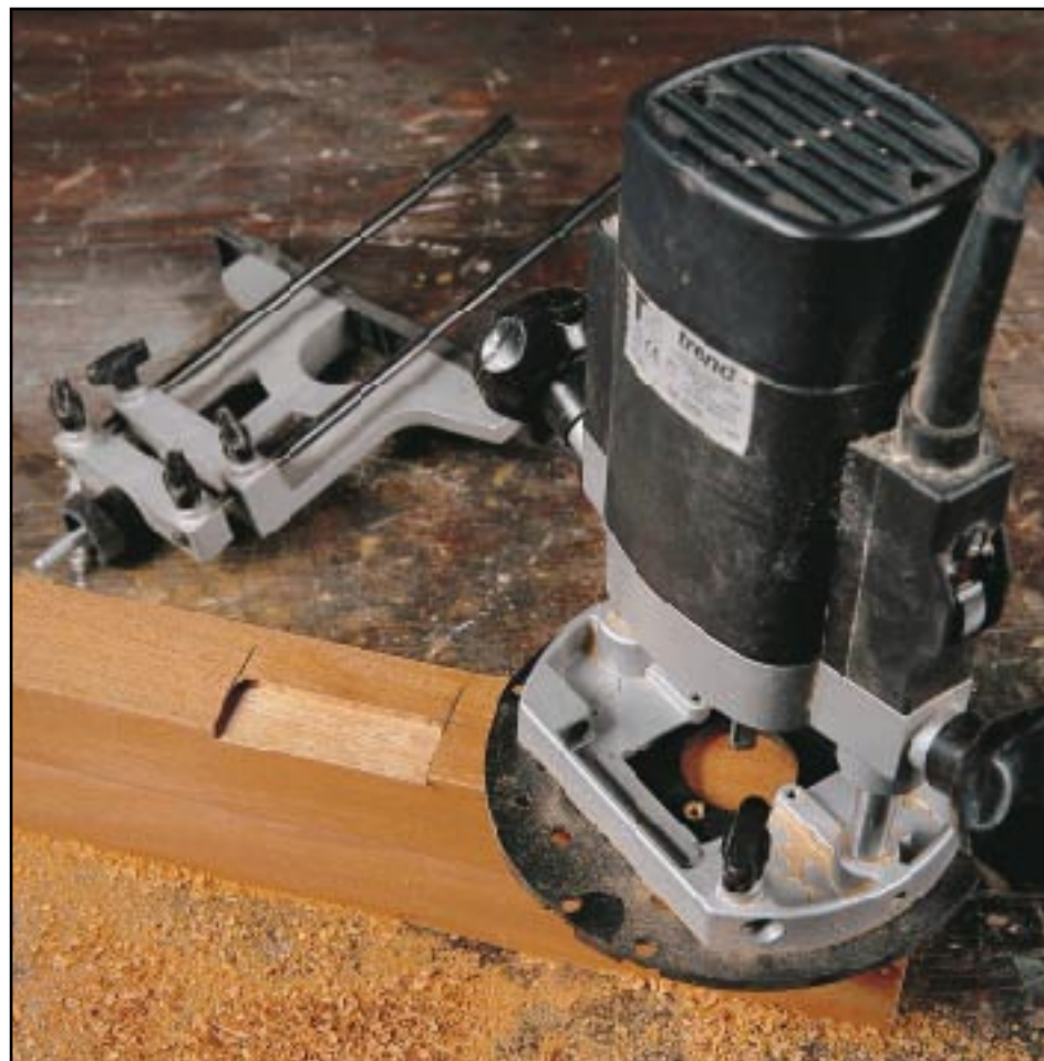
◀ The Unibase stops a small router dropping into a large hinge recess
