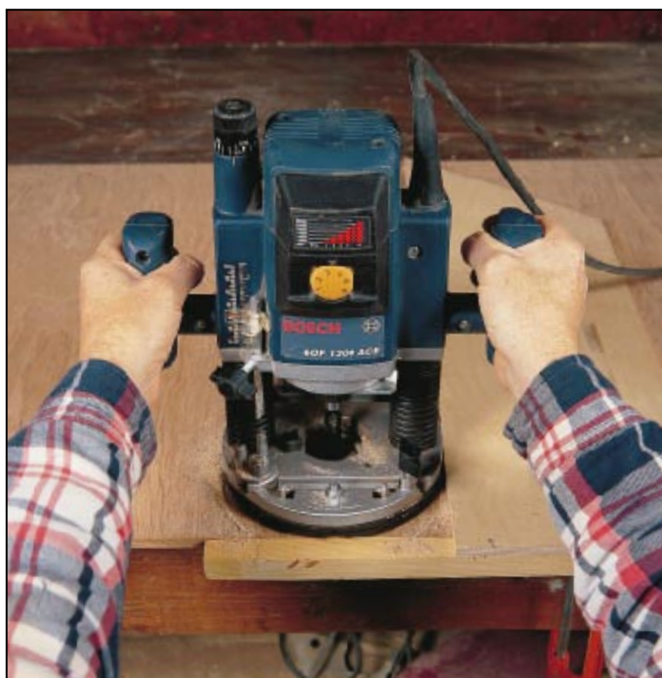
▶ Exact cutter-to-fence distances are possible with Unibase
