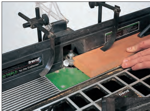
Cutting the edge profile on the trial piece
