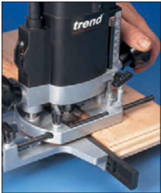
Edge moulding using a side fence.
